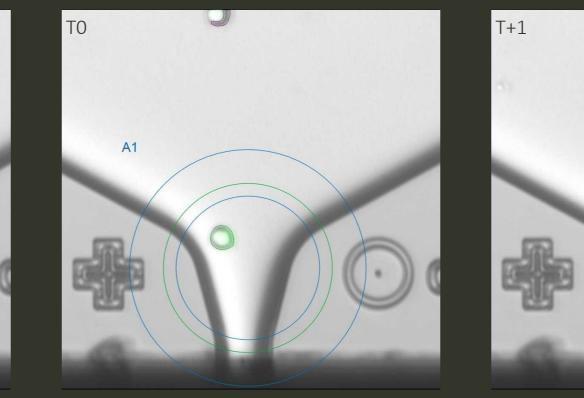
EXAMPLE OF UP.SIGHT™ NOZZLE IMAGES DURING CELL DISPENSING Series of images (overlay of brightfield and fluorescent) taken during dispensing of GFP-expressing iPSCs, T0 indicates recognition of the cell, T+1 shows the
