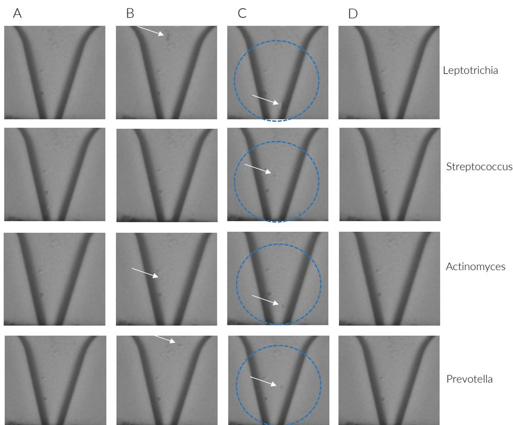
**Figure 2.** B.SIGHT nozzle images showing the isolation of a single microbial cell. The cell approaches the nozzle (**A, B**). The cell is detected in the nozzle by the automatic image processing algorithm (**C**). Image **D** shows the empty nozzle after the droplet with the single cell was dispensed.
