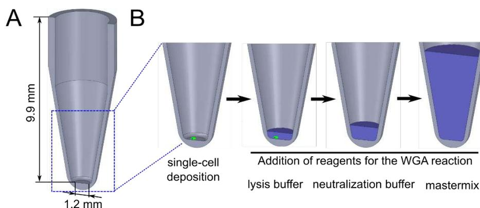
**Figure 3.** Precise dispensing of a single cell into conical PCR plates. Plate deionization to remove electrostatic charges and the automated offset correction (AOC) module enable the deposition of a single cell (green sphere) onto the bottom of the well (A) as a prerequisite for the lysis and WGA in miniaturized volumes (B).
